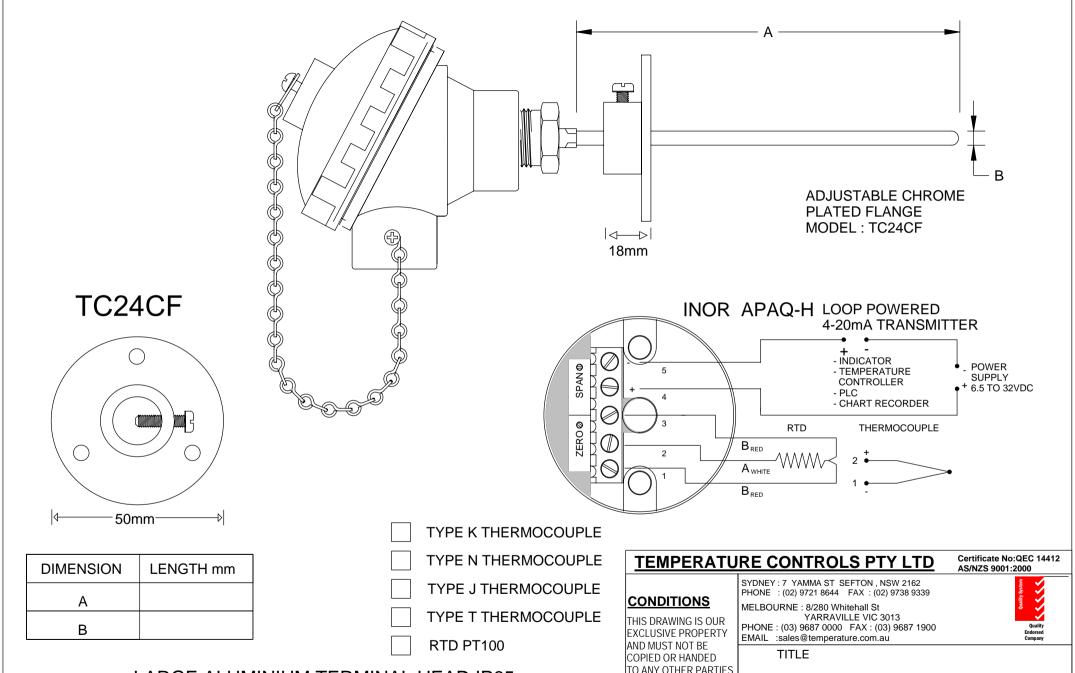
LARGE ALUMINIUM TERMINAL HEAD IP65 4-20mA TRANSMITTER NON ISOLATED RANGE: (AS SPECIFIED)
